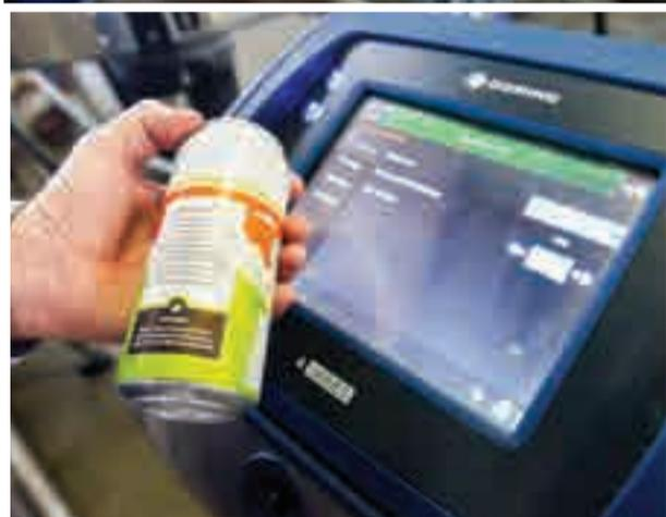
The Domino model A201i continuous inkjet printer is used to apply production date codes onto the bottom part of the filled aluminum beer-cans.
